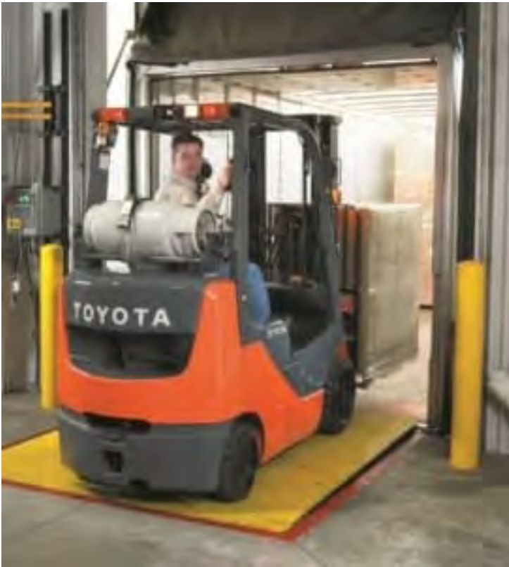
Exhibit 2-9: Forklift on Loading Dock - Dock Leveler
