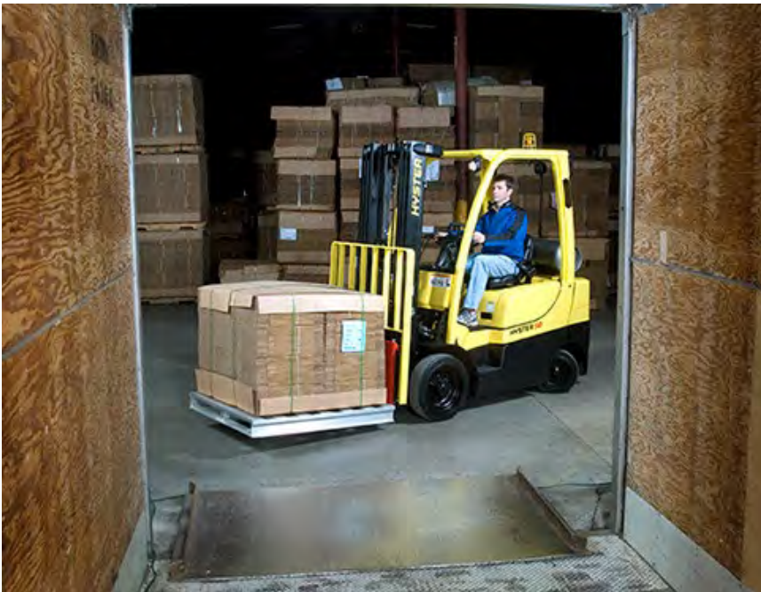
Exhibit 2-7: Forklift on Loading Dock - Bridge Plate
