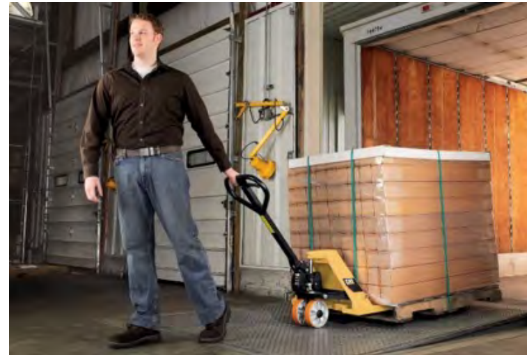
Exhibit 2-6: Pallet Jack on Loading Dock
