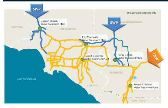
Physical and operational changes being made to the distribution system to preserve limited State Water Project Supplies
