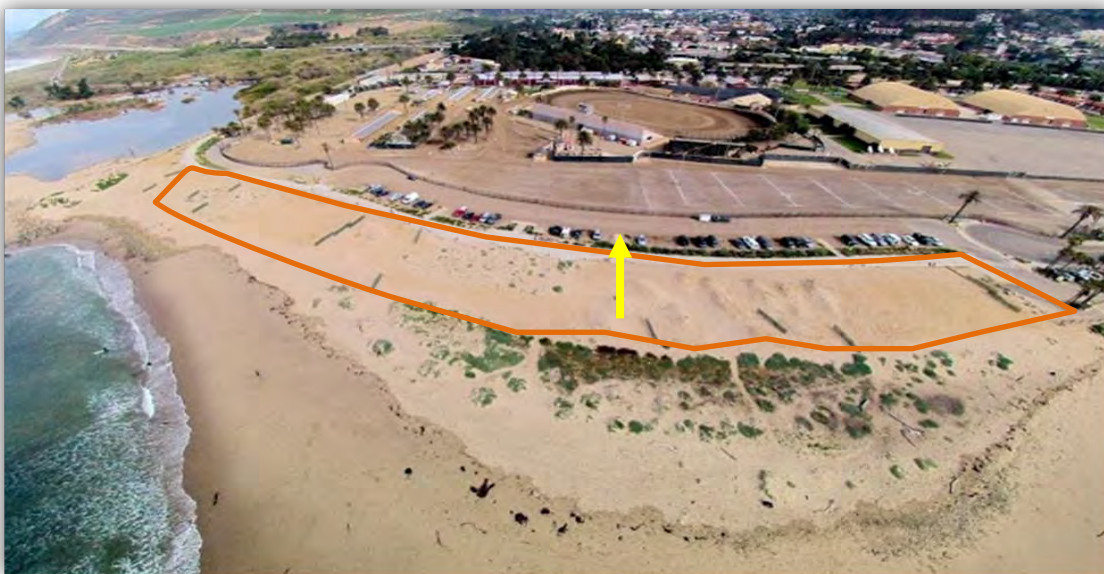
Figure 16. Photo depicting “managed retreat” and restoration. Surfers' Point Managed Shoreline Retreat project in which the parking lot was moved back and beach area was restored. (Aerial composite by Rick Wilborne (February 28, 2013); photo courtesy of Surfrider Foundation)
