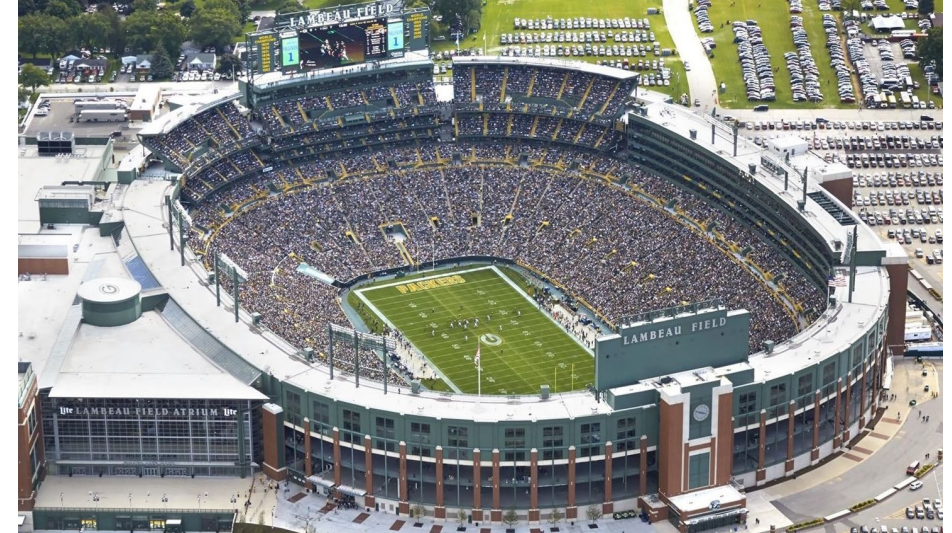
Avg. NFL Stadium = 5-10 MW
