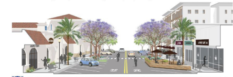
D A Street (3rd St to 7th St): Back-in angled parking, landscape enhancements at mid-block crosswalks, bike corrals, and parklets can add life to A Street's retail environment.
