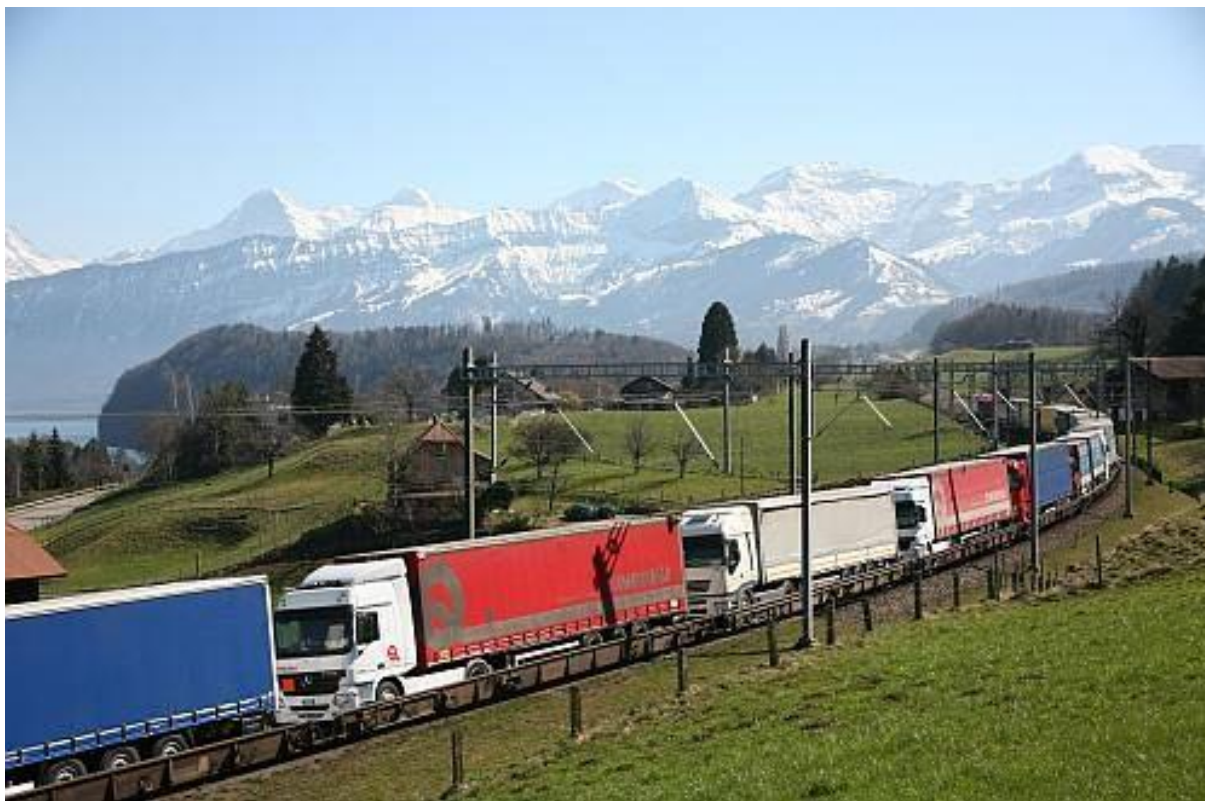
RAIpin 'rolling road' electric train carrying trucks in Switzerland
