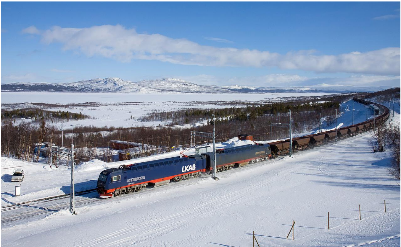
Fig. 1. Bombardier IORE electric locomotive set hauling an iron ore train between Sweden and Norway
