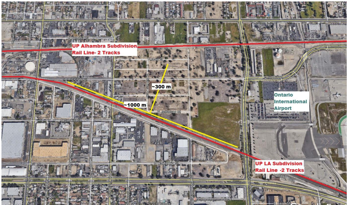
Fig 15. Possible “All-Electric Ontario Intermodal Facility” site, with dimensions (Background aerial photo: Google Earth)
