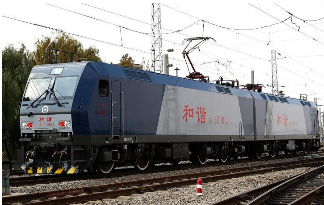
Fig. 2. China Railways HXD1 series freight locomotive set, under 25 kV overhead catenary wire (Photo: https://commons.wikimedia.org/wiki/File:HXD10004.jpg )
