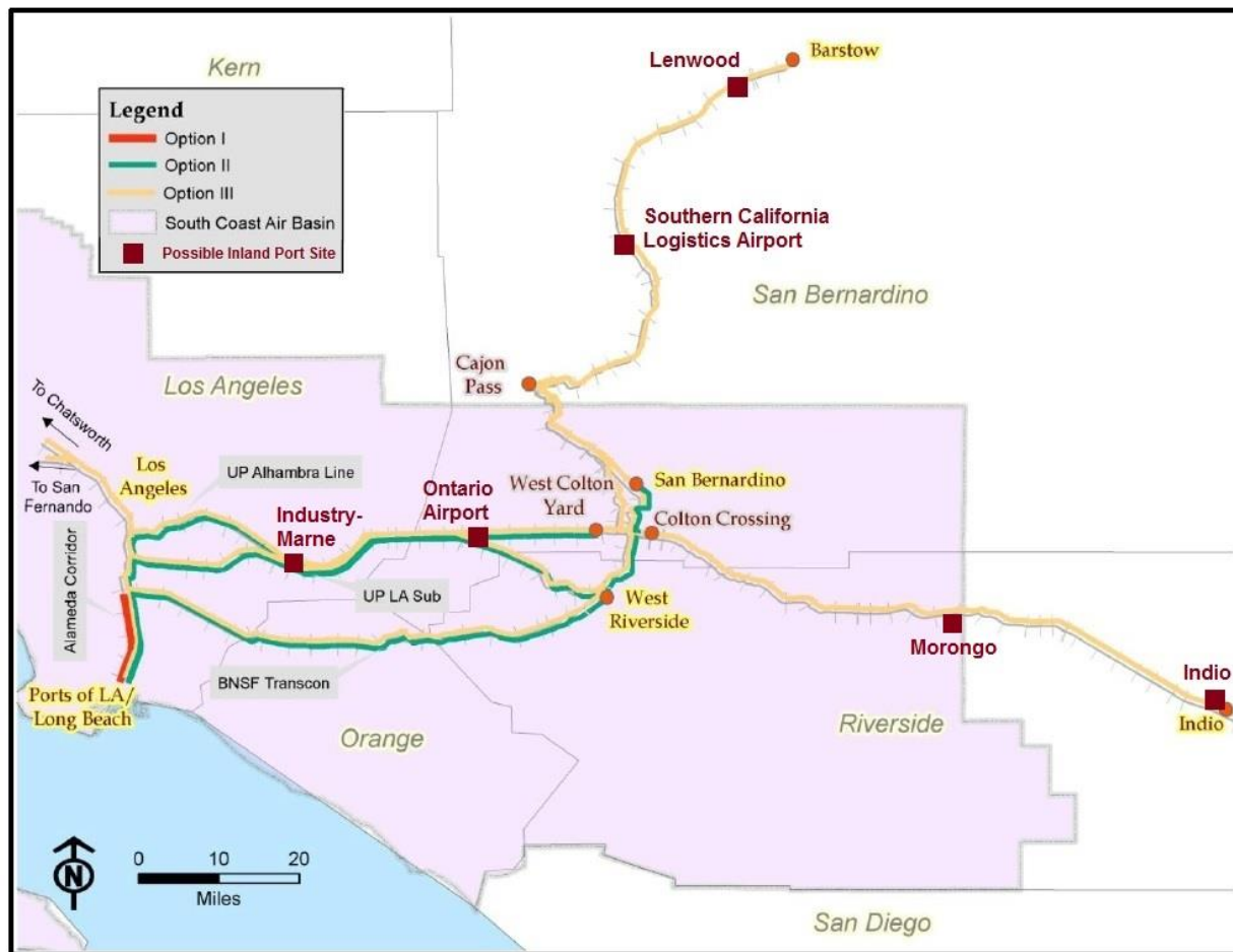
Fig. 10. Freight rail electrification scenarios in the South Coast Air Basin, as proposed by 2012 SCAG report, and annotated to show possible intermodal facility sites for electrified short-haul rail service.
