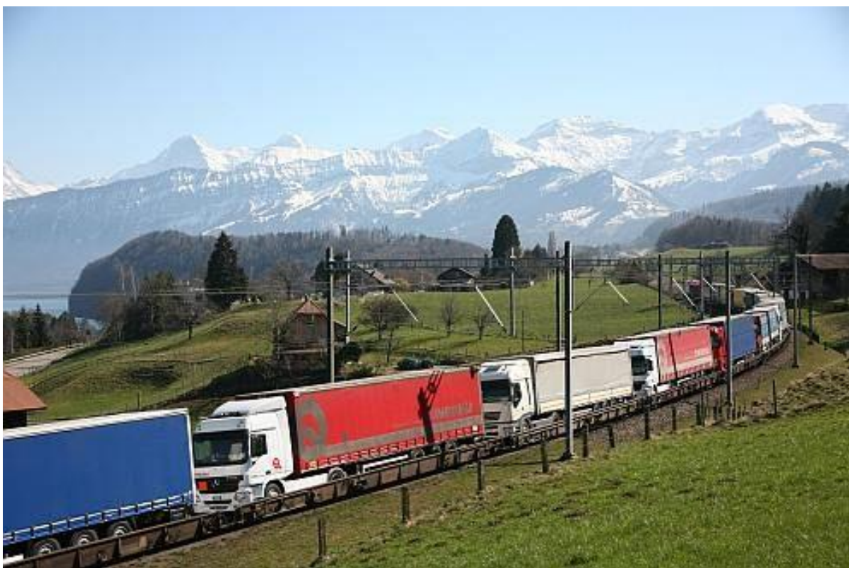
Fig. 11. RAlpin ‘rolling road’ electric train carrying trucks in Switzerland (Photo: RAlpin AG, http://www.ralpin.ch/media/ )
