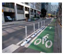
**Class IV Separated Bikeway** A Class IV separated bikeway is a cycle track or protected bike lane that is physically separated from vehicular traffic using bollards, planters, or parked automobiles.
