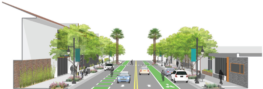
a A Street (Deodar Ave to 3rd St): New bike lanes (either colored green as shown or simply striped with white paint) along with new street trees in existing empty tree planters, new pedestrian-scale street lights, and new mid-block crosswalk with curb extensions and palm trees to mark the crossing. Such improvements could surely be made in phases, as funding allows.
