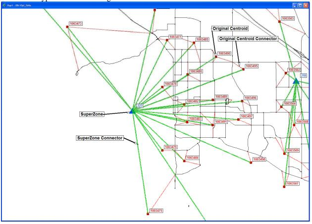
In the above diagram, there is one superzone connector link between the superzone node and each TAZ node within the superzone. The superzone nodes are numbered between 1 and the highest superzone number. As the illustration also shows, the original regional network centroid nodes have been renumbered so that they reflect the original centroid node TAZ number plus 1,000,000. Again, the superzones, connectors, and renumbering of original zones only occur in the areas that are aggregated.
