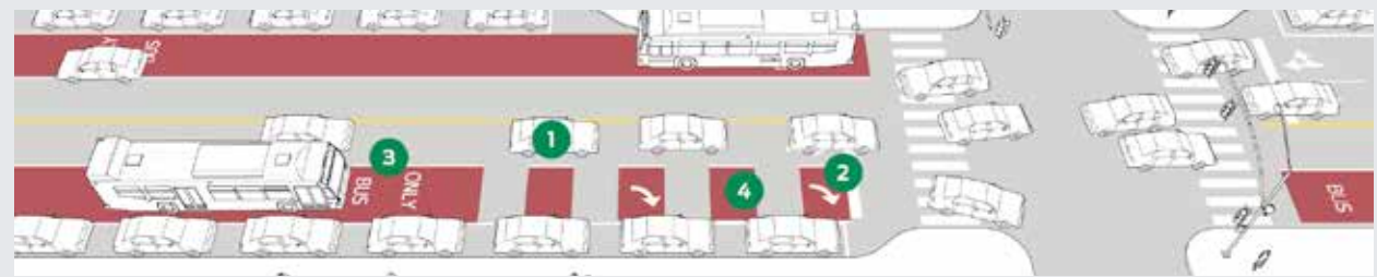
Transit Approach Lane (top) and Queue Bypass (bottom); green numbers highlight pavement marking features. Source: NACTO Top: https://nacto.org/publication/transit-street-design-guide/intersections/intersection-design/transit-approach-lane/ Bottom: https://nacto.org/publication/transit-street-design-guide/intersections/intersection-design/shared-right-turn-lane/
