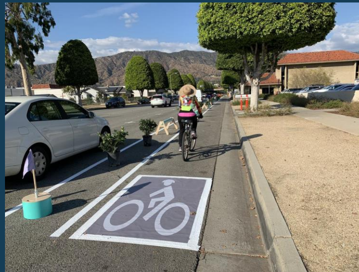
Example of separated bike lane
